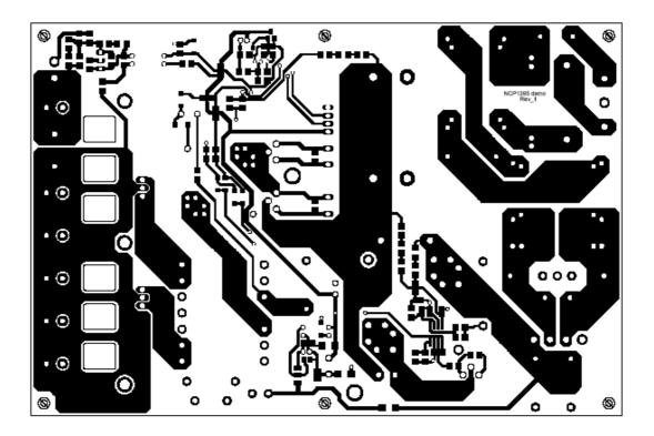
Figure 27. Bottom Side (Bottom View)
