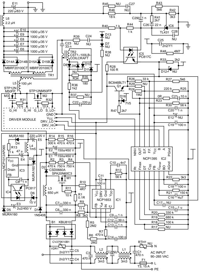
Figure 1. Schematic of the NCP1395 Demo Board
