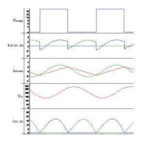
Figure 8. Typical waveforms of the LLC converter operating in the 2<sup>nd</sup> area of the gain characteristic.
