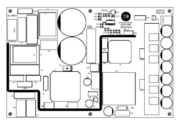
Figure 24. Component Placement on the Top Side (Top View)
