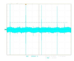
Figure 18. Output Ripple Under Full Load
