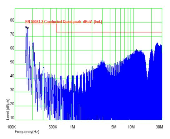
Figure 23. Conducted EMI Signature of the Board
