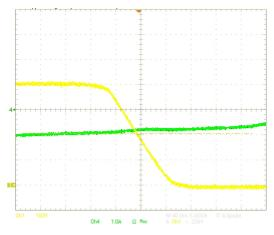
Figure 16. Detail of the ZVS Condition – Falling Edge
