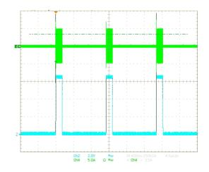
Figure 20. Operating Under Short Circuit
