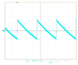
Figure 19. Output Ripple During the Skip Mode
