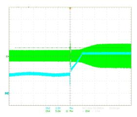
Figure 21. Full Load to Short Circuit Transition
