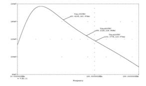
Figure 10. Simulated Gain Characteristic of Proposed LLC Converter – Full Load Conditions
