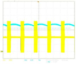
Figure 22. Operation in the Skip Mode
