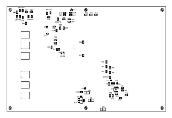
Figure 26. Component Placement on the Bottom Side (Bottom View)
