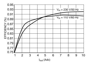
Figure 11. Efficiency of the Designed Converter versus Output Current
