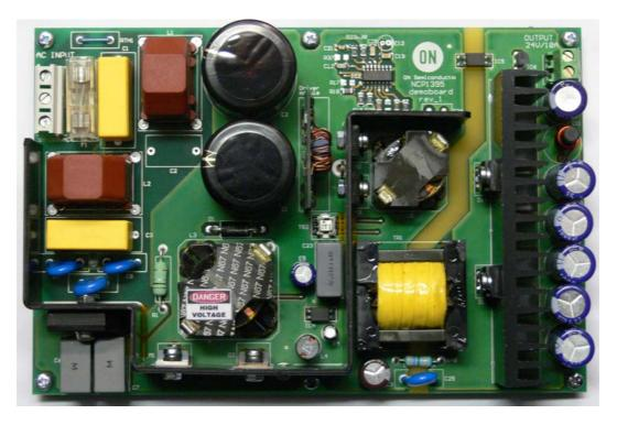
Figure 28. Photo of the Designed Prototype (Real Dimensions are 183 x 122 mm)
